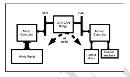
Two or more segments can be connected by repeater or bridge devices as shown in the diagram below.
